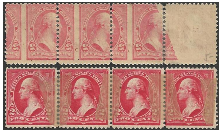
Figure 3. Reverse offset on a stamp printed on a flat plate press.
