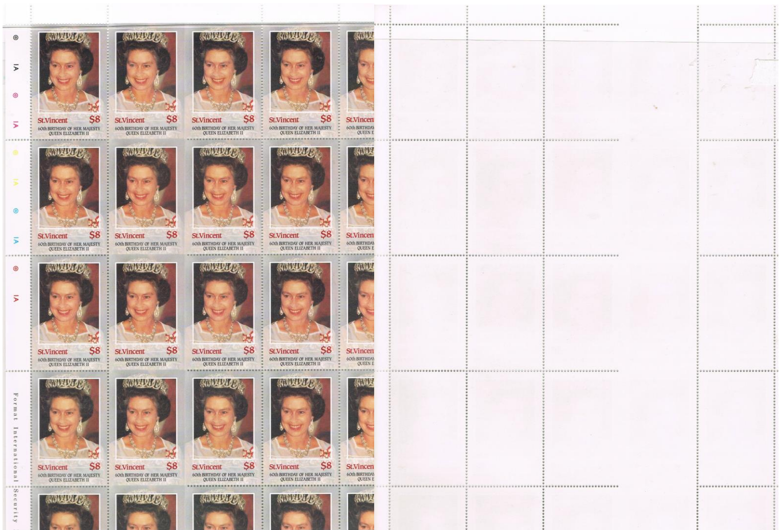
GB has long used comb perforations, starting with the first stamps. This St. Vincent sheet was printed in the UK. It shows a skipped row of perforations, courtesy of John Hotchner.
